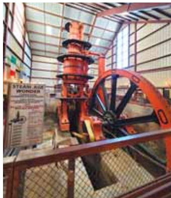
Running "full steam," the engine could pump more than 4.59 million gal in 24 hr.
