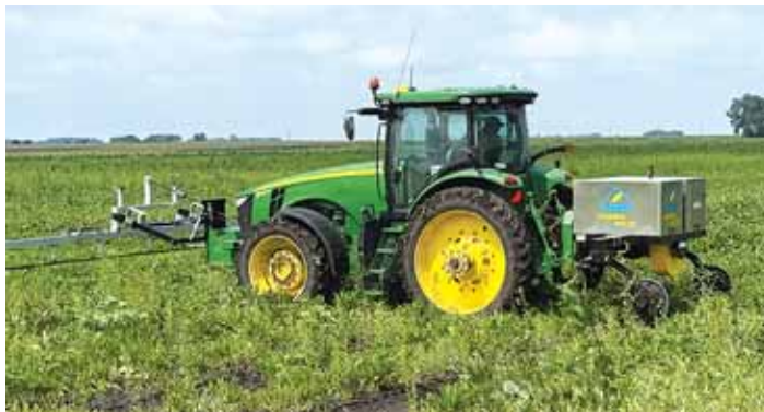
Early Lightning Weeders were limited to a 24-ft applicator bar, but advances now allow up to 44 ft of coverage from a single generator.
