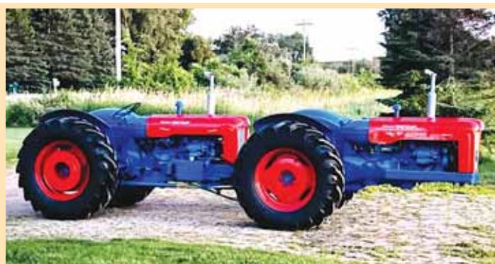
Tractors are joined by a pivot frame resembling a lazy Susan on the rear of the front tractor.
