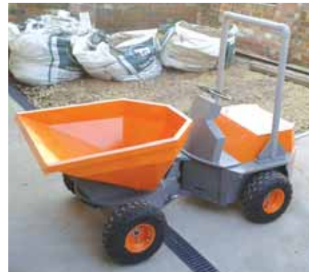
Dumper pushcart is made of marine-grade plywood with an aluminum-reinforced center-pivot.
