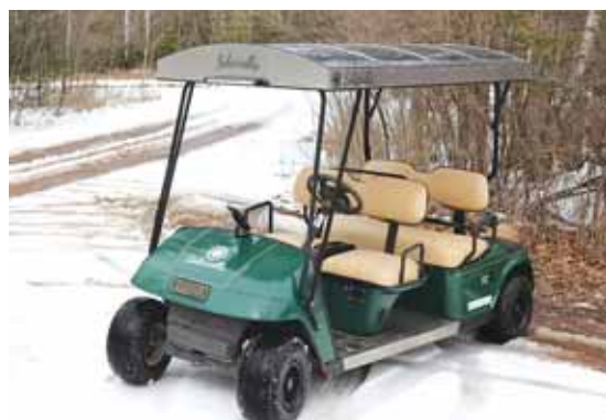
Converting older golf carts into solar utility vehicles is a major part of the business. They handle custom projects and convert some for sale.
