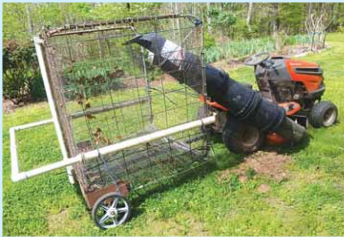
Reid made the entire leaf transfer ducting from nested 5-gal. plastic buckets.
