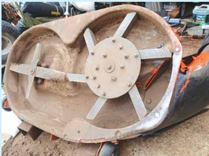
Reid designed an impeller blade to replace the lawn mower blade. It’s a 10-in. dia. steel plate with six angle-iron blades bolted to it, providing a 22-in. dia. cut.
