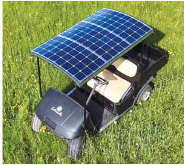
“We make a dedicated, semi-flexible solar panel for the golf carts,” says Balan. “It’s precisely engineered to weigh around 30 lbs.”
