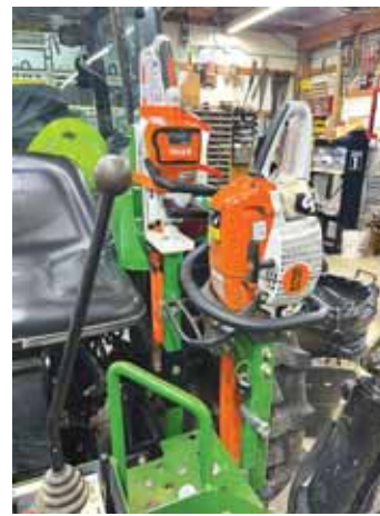
"Using the receiver hitch concept for the chainsaw holders makes it easy to duplicate on other pieces of equipment where a chainsaw, log chains or other tools can come in handy," says Freeman.
