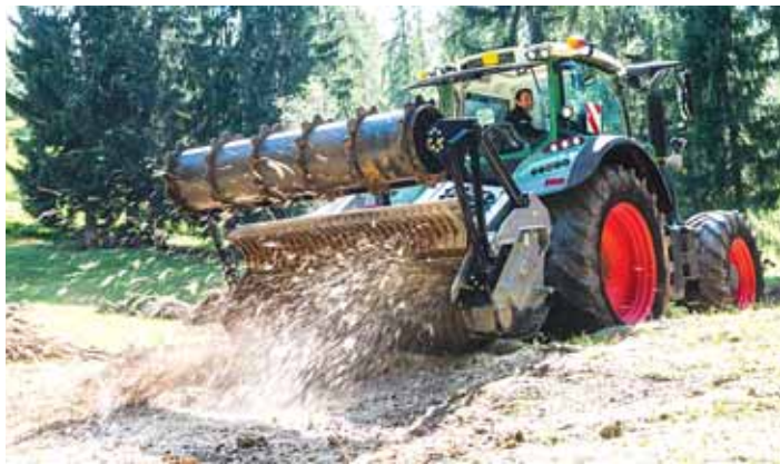
“FAE multitask heads are highly valuable in agricultural applications,” says FAE Group Marketing Specialist Kevin Warstadt. “They can be used to clear land for planting, remove stones, roots and stumps, and eliminate leftover debris after harvests.”
