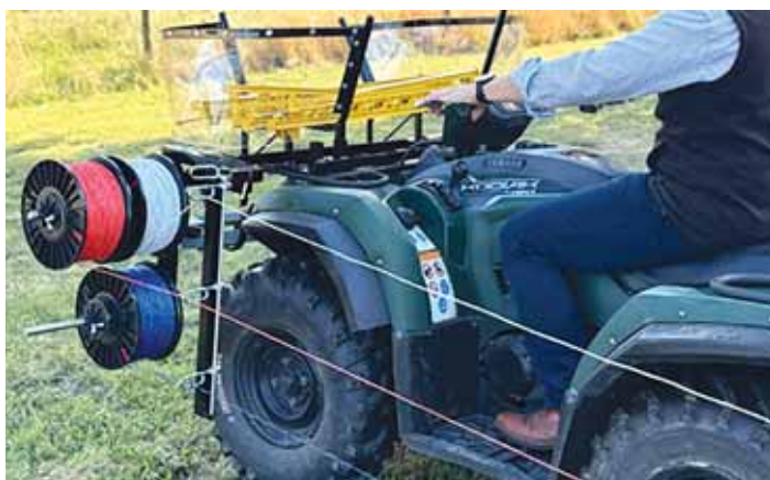
Unwinder mounts to the front of an ATV to easily unwind fence lines without tangling or twisting.
