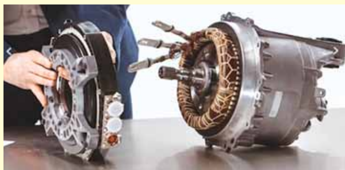
Similar output axial flux (left) and radial flux (right) electric motors.
