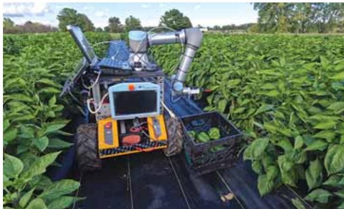
Kim used a custom handheld shear-gripper with sensors to teach the robot to pick peppers by mimicking human actions and using advanced software.
