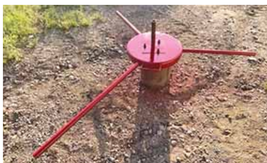
Gutschmidt welded handles onto the bases so they can be carried like suitcases once the outrigger pipes are removed.
