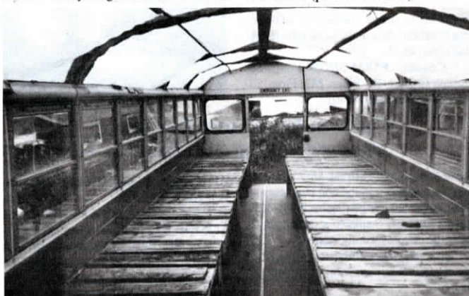
There are two layers of poly on top of bus, which has room for 75 flats and 50 hanging baskets.
