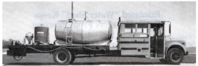
After a little work, 1975 schoolbus makes handy nurse tank for spraying.
