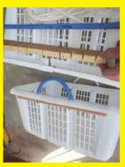
I repaired my wife's laundry basket using two oak boards (3/4 in. by 1 1/2 in. by 16 3/4 in. long), two 1/2-in. PEX pipes (10 in. long) and two 1/4-in. dia. nylon ropes (20 in. long). First, I rounded off one edge of the boards. Then I cut 3/4-in. deep slots to accommodate the plastic gussets. Finally, I drilled 1/4-in. holes 6 in. apart.
