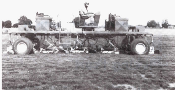
Both wheels and driver pivot to drive machine lengthwise.
