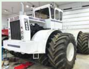
Brecka and his son rebuilt the 1978 KT 450 Big Bud's stock Cummins 1,150-cu. in. engine plus the transmission.
