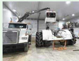
Brecka and his son rebuilt the 1978 KT 450 Big Bud's stock Cummins 1,150-cu. in. engine plus the transmission.
