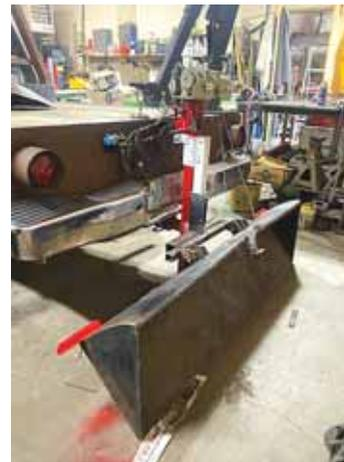
Heron's bucket is powered by an electric winch.
