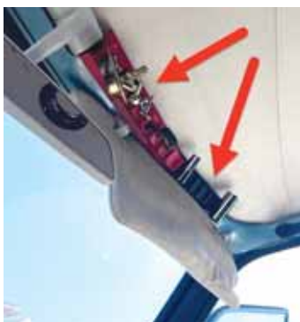
Sturdy magnetic straps hold sockets and tools close at hand.
