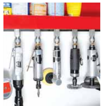
Tool holders quick connect to hold air tools in place and keep connections clean.
