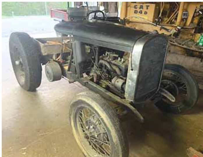
Schraner's family tractor uses a 1931 Model A Ford 4-cyl. gas engine.
