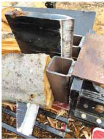
Hawkes used steel tubing for the long blocks. The gap left between them accommodated the vertical wedge, extending the reach of the horizontal wedge.
