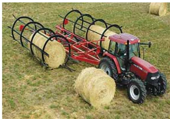
Each chamber is equipped with floating springs, which make them virtually weightless as they contact the ground.
