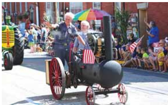
Dryden built a small yet authentic-looking parade-ready custom steam engine out of rusty farm parts and a Fairbanks Morse Z gasoline engine.
