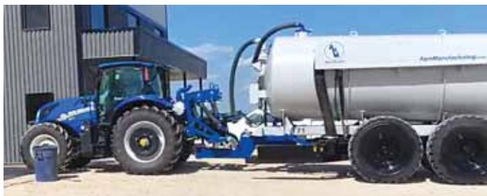
Rather than coupling the tank's PTO drive to the tractor before each use, the main hose is connected to the rear of the pump. As the tractor completes sharp corners, the hose moves freely as it slides back and forth.
