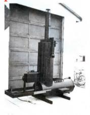
When the vertical chamber fills up with cans, glass and ash, the bottom compactor is used to empty it.
