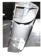
Moisture sensor straps to combine's clean grain auger. A metal "fin" extends inside to take readings off grain passing over it.
