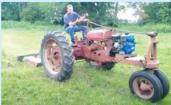
“The clutch plate eye conversion can let you connect almost any manual transmission to any motor,” says Floerkey.
