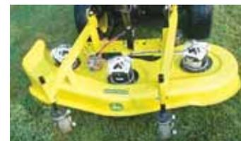
Mower deck stays parallel to the ground when lifted.
