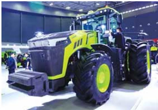
The company isn't sharing too many details but hints that using an electric power boost lowers the tractor's fuel consumption by approximately 8%.
