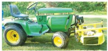
Bertalotto used three 40-volt Craftsman electric lawn mower motors when converting a belly mount mower to front-mount.
