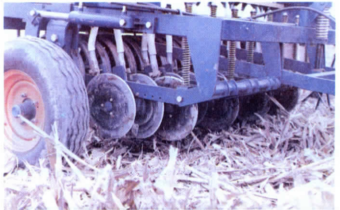
Precision depth control is key feature of 7 ft. wide Moore drill which plants 18 rows spaced 4 3/4 in. apart.
