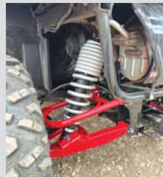
Orwick praises the long-travel double-wishbone front and rear suspension.
