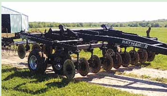
Preul cut the wings off one of the units to use only the center section. He spaced the 17 20 1/2-in. fluted opener blades from the two applicators at 9-in. centers.
