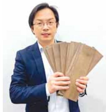
Superwood is five times thinner, but has four times the density of wood. It's 4 to 20 times stronger.
