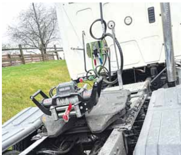
Adapter goes from the 5th wheel kingpin to a 2-in. receiver hitch.
