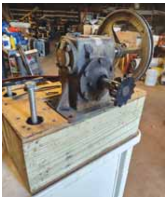
"I started with an old 50:1 gear head, powered by a residential garage opener," says Harmon.
