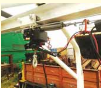
Winch and cable trolley allow for easy lifting and hauling of large items.
