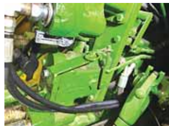
Glanville created a small device to hold his tractor's hydraulic levers in constant down pressure and lock the valve in the operating position.
