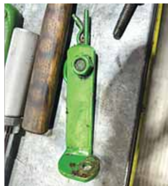
Device consists of a 5-in. long and 3/16-in. thick piece of flat iron welded at a right angle.
