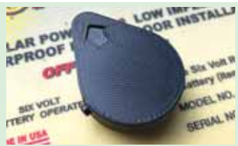
Steffen created a replacement knob complete with a small set screw to securely attach it to the fencer and an arrow to clearly indicate the on or off status.
