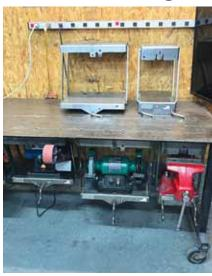
The Tool Swing easily swings up a vise, bench grinder, sander, chop saw or other tool, then quickly unlatches and swings it out of your way.
