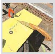
John Rochester, Charlotte, N.C.: "A clamp and a washer can be used to prevent a cut from dropping down and splitting. This works for bigger stuff using a piece of wood.
