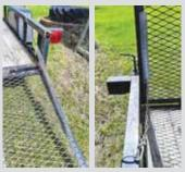
"A couple of springs, short pieces of chain, and U-bolts made a simple, inexpensive lift assist for my trailer tailgate."
