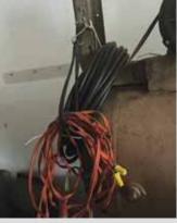
"Rubber bungee cords, hooked where convenient, make great, easy-to-use hangers for cords and hoses. Just attach the bottom hook to the top hook.
