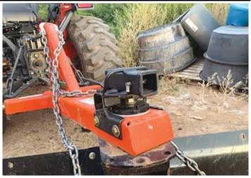
Buckner cut down a receiver hitch, then used mounting brackets to fit it around the scraper's pivot.
