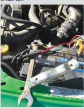
"To ground a vehicle battery to the frame, connect the negative terminal of the battery to the vehicle's frame using a wrench and metal clamp, making sure the connection is tight and free of corrosion. This allows the electrical current to flow properly throughout the vehicle's electrical system.
