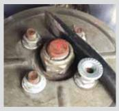
"Sometimes, it can be hard to loosen a nut. This photo shows the friction-drive wheel on a rear-engine Snapper rider. To keep the pry bar on the studs while loosening the nuts, reverse a flange nut and turn it over to create a shoulder. The bar won't slide off the studs now."
