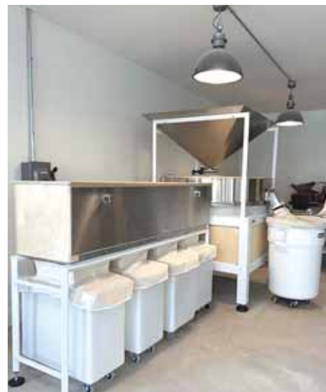
New American Stone Mills 40-in. mill with sifter.
