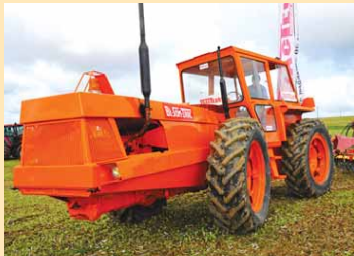
Bi Som Trac was a French tractor with a single engine and four drive wheels, a design that evolved from two Someca 40 tractors hooked in tandem.
