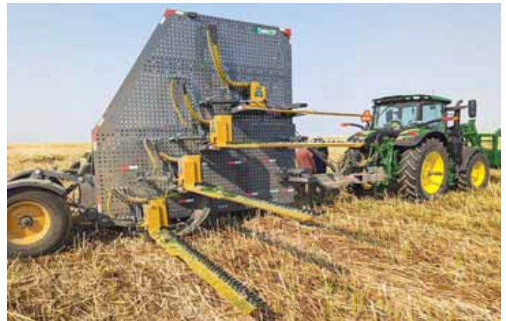
FiberCut operates at speeds up to 15 mph, cutting tall stalks into manageable 27 to 78 in. sections.
