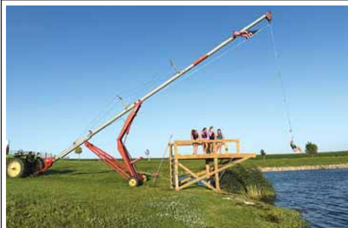
Bonnema hitched the auger to his Deere 3020 tractor and used the hydraulics to raise it for swinging at any height and to lower it if the winds were too strong.
