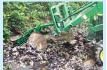
Creek rake has no hydraulics, and is used by tilting loader and moving tractor forward and back.
