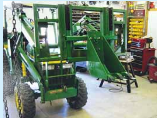
Stump puller's 2 by 2 in. steel tube frame mounts directly to unibracket for maximum torque.
