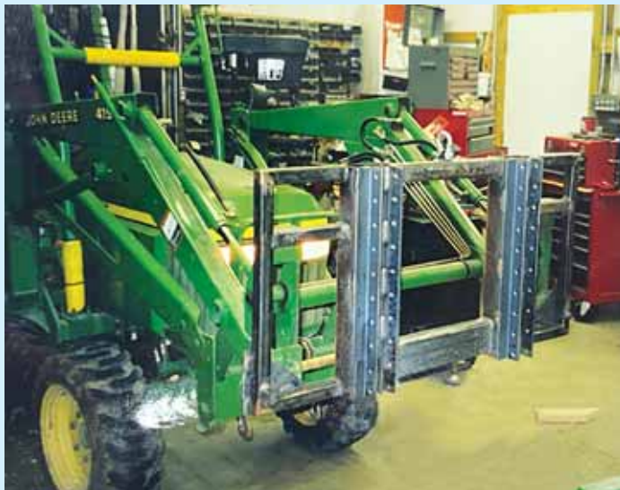
25 by 50 in. unibracket with vertical angle irons drilled top to bottom for attachments.
