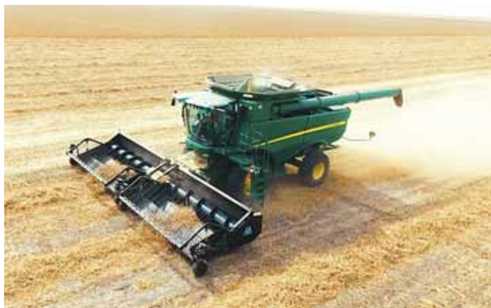
Double header features an advanced floating suspension system that adjusts to uneven ground and is designed to minimize seed loss.
