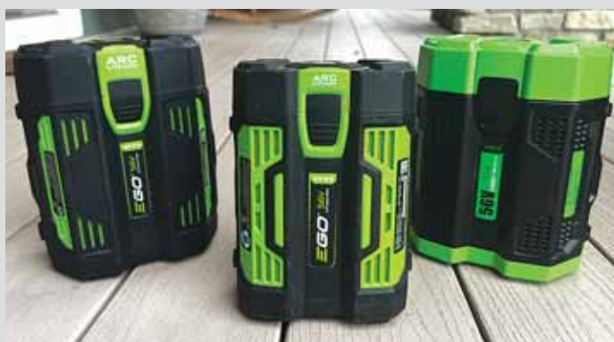
OEM 56V 5Ah battery shown on left, 2.5Ah battery in middle, and non-OEM 5Ah battery on right.
