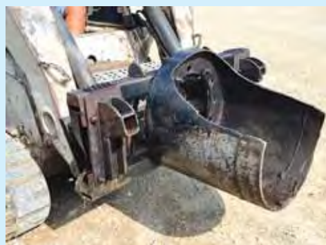
Hernke cut away half of an old 25-in. dia. rim from a Terragator, then bolted it to an old skid steer frame to make a dandy tree spade.
