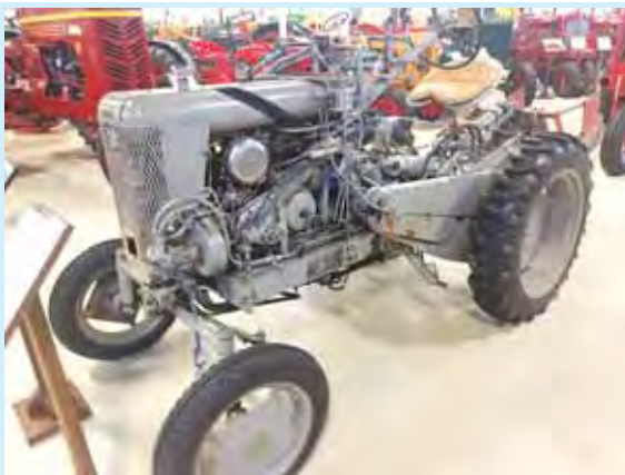
One-of-a-kind tractor powered by a WWII Indian motorcycle motor.
