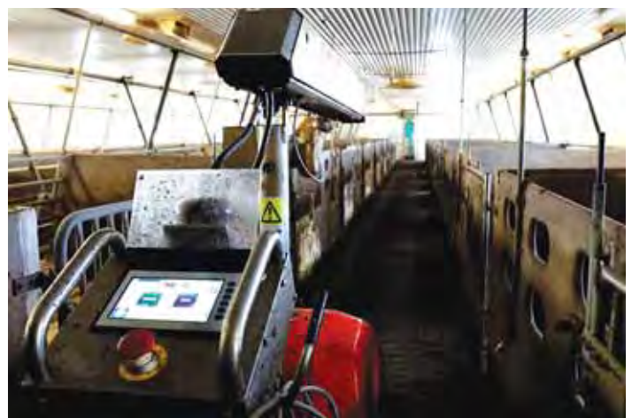
Robot's arm extends about 19 1/2 ft. and moves the wand 180 degrees. The spray tip rotates 360 degrees to reach every corner.
