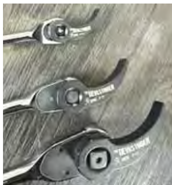
Redesigned tool works with a 4-pt. drive and has flattened sides, making it easier to use with a wrench or pliers.
