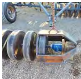
Open-to-the-bottom puller has three 1-in. thick side and top pieces welded together.
