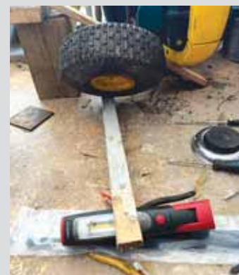
John Rochester, Charlotte, N.C.: "To make it easier to install a tire, I use a board with something under the far end to get it to the right height so I can install the washer and cotter pin without having to try to hold up the wheel at the same time."
