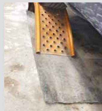
Keith Peterson, Moorland, Iowa: "When using car ramps, I cut a piece of material about a foot longer than the car ramp and set the ramp on top of it to keep it from moving around."
