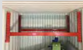
Pat Hiebert, Victoria, B.C.: "I made a shelf using some old skid racking. I cut the racking to length and ensured that the vertical uprights were lined up and straight before cutting. I welded hooks to the top and now have a shelf I can park motorcycles under."
