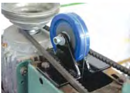
Foale added a cylinder counterweight inside the column of his Startrite drill press, running a cable across a pulley and down to the table, making it easier to raise and lower.
