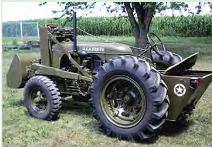
Case SI was a downsized version of a Case SC, featuring different fenders and a distinct front and rear end. Loops on each axle were used to secure the tractor during flight.
