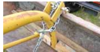
Loader mount chain wrap and wood stabilizers.
