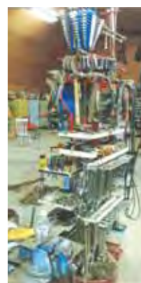
Tool "tree" was built with an old New Holland baler flywheel as a base. Haubrich attached a section of 2-in. square tubing as a support post and added what he needed around the center.
