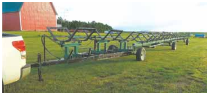
Old swather beam used as the key piece of a trailer that holds nine round bales. Haubrich added metal bale cradles and hooked them up to dump hydraulically.
