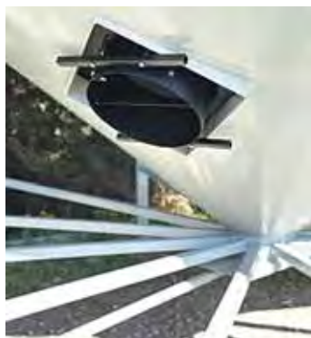
Wavcor Manhole attachment includes a round or square plate that slides inside standard bins' 21 or 24-in. manholes, along with a double-bar system with three bolts for installation or removal of the attachment.
