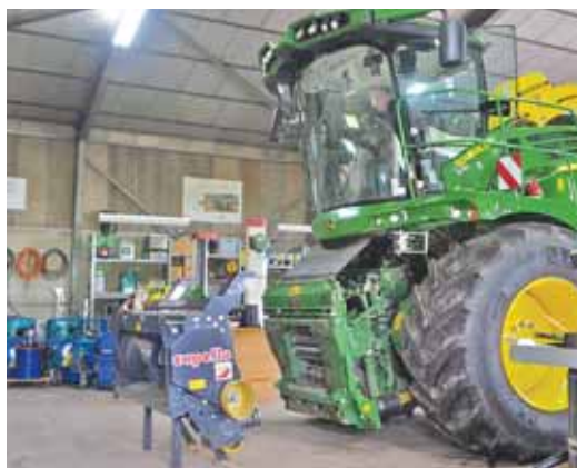
With the module in place, the forage harvester attaches to the Capello corn header just as it would with a combine.
