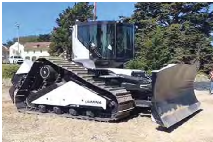
Moonlander ML6 all-electric, 750-hp, 32-ton bulldozer.
