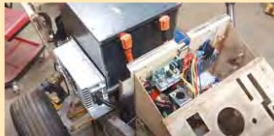
Electronic components are stored in their own compartment beneath the dash panel.
