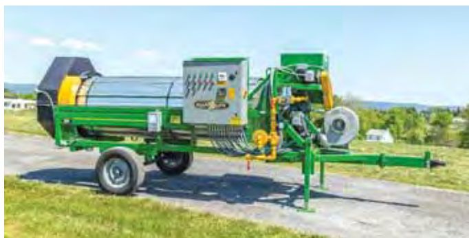
Roasters are powered by propane and electricity. The grain is augered into the roasting drum, then moves to the cooler before being loaded into a truck, wagon or storage bin.
